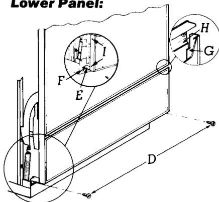
1. Remove two screws (D) located under panel.
