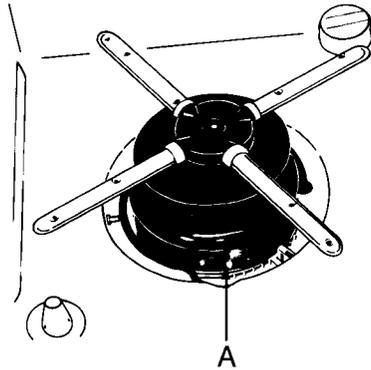
TO REMOVE the stainless steel filter, lift lower wash arm straight up. Lift filter out. TO CLEAN, scrub with a stiff brush under running water. TO REPLACE, snap stainless steel filter over the ultra-fine filter and then replace wash arm. When replacing wash arm, be sure that water jets are facing up.
