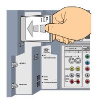
Inserting the CableCARD incorrectly may result in permanent damage to the card and
