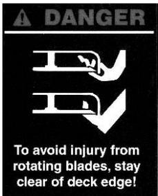
Keep hands and feet clear of the deck edge. Never reach under the mower deck until the blades have come to a complete stop.
