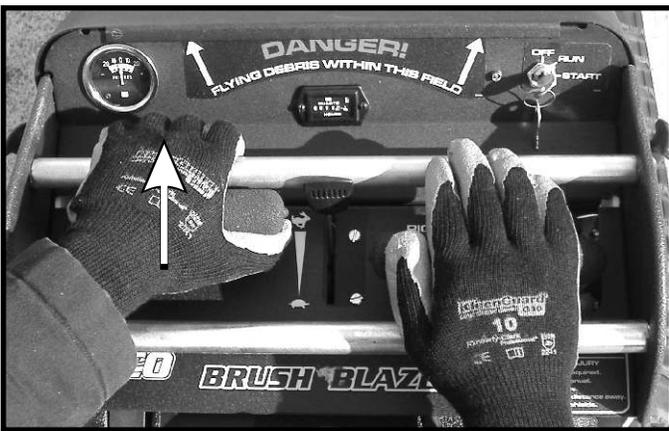
Keep your right hand on the right steering control handle. Grab the left steering control handle with your left hand and push forward to steer right. Push the control forward slightly to steer slowly. Pushing the control harder will execute a sharper turn.
