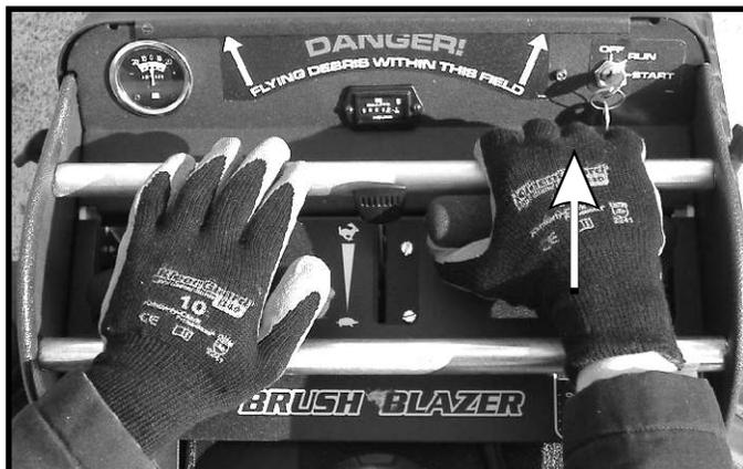
Keep your left hand on the left steering control handle. Push the right steering control handle forward to steer to the left. Push the right steering control slightly to steer slowly. Pushing the control harder will execute a sharper turn.
