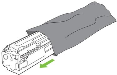
5. Remove the orange, plastic shield from the bottom of the new print cartridge.
