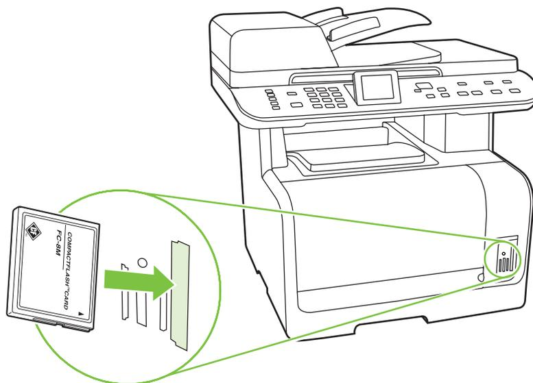
2. The product reads the card, and then the product control panel displays **X photos found on card**, where X is the number of recognized .JPEG files found on the memory card.
