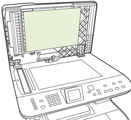
3. Also, clean the scanner strip next to the ADF scanner glass.
