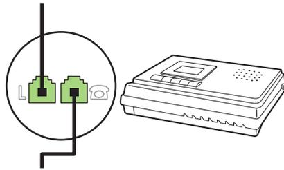
7. To connect a telephone, plug a telephone cord into the previous device's "telephone" port. Plug the other end of the telephone cord into the telephone "line" port (also called Faxtel).
