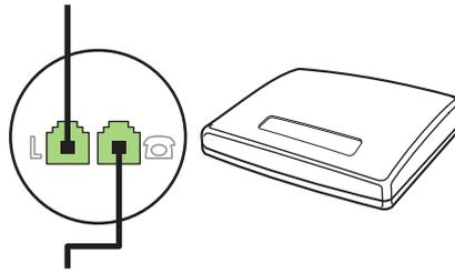
6. To connect an answering machine, plug a telephone cord into the previous device's "telephone" port. Plug the other end of the telephone cord into the answering machine "line" port (also called a TAM).
