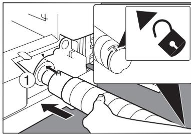
① Align the Key of the bottle, also represented by the Arrow mark (**Unlocked** symbol
