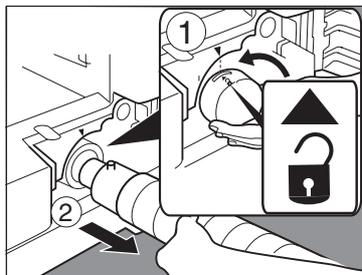
① Turn the empty Toner Bottle counter-clockwise until it stops. The Arrow mark (**Unlocked** symbol 🗝️) visible on the end of the Toner Bottle is aligned with the Arrow mark on the machine.
