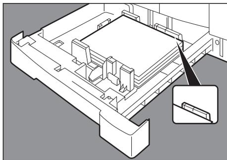
Make sure paper is not loaded above the overfill indicator located in the Paper Tray.
