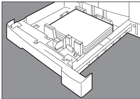
Place the paper with the copying surface facing upward.
