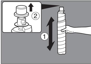
① Shake the new Toner Bottle four or five times to loosen the contents.
