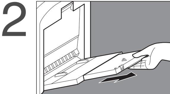
Pull out the sheet bypass tray until it stops.
