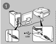
Connect one end of the USB cable to the computer and the other to the machine.
