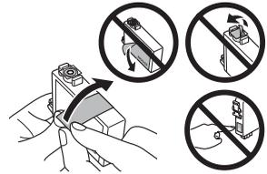
7. Insert the new ink cartridge into the holder and push it down until it clicks into place.
