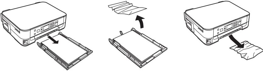
2. Lift the scanner and carefully remove any paper trapped inside.
