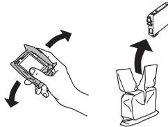
6. Remove the yellow tape from the bottom of the ink cartridge.
