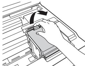
4. Squeeze the tab on the cartridge and lift it up. Dispose of it carefully. Do not take the used cartridge apart or try to refill it.
