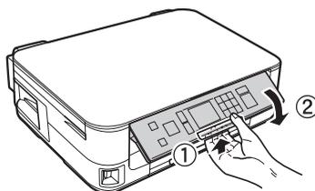
**Caution:** To avoid damaging your product, always squeeze the release bar to lower the control panel.
