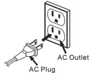
NOTE: This system is equipped with a polarized AC power plug having one blade wider than the other. This is a safety feature. If this plug does not fit into your existing AC outlet, do not try to defeat this safety feature by filing the wide blade to make it fit into your outlet.
