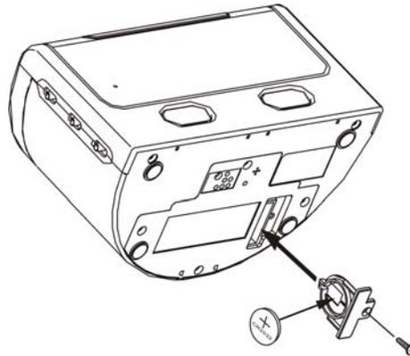
4. Remove the original battery from the holder and insert the new battery into the holder the same way, observing the positive (+) direction. Slide the holder with the new battery back into the slot in the cabinet.
