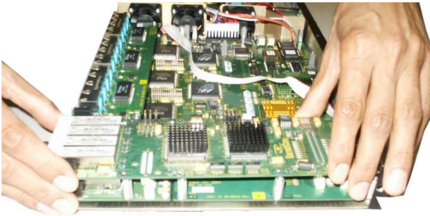
Fig 3.5.2e Daughter Bd. Being placed over the Grand daughter Bd. and the mating connector being matched to lockup properly
