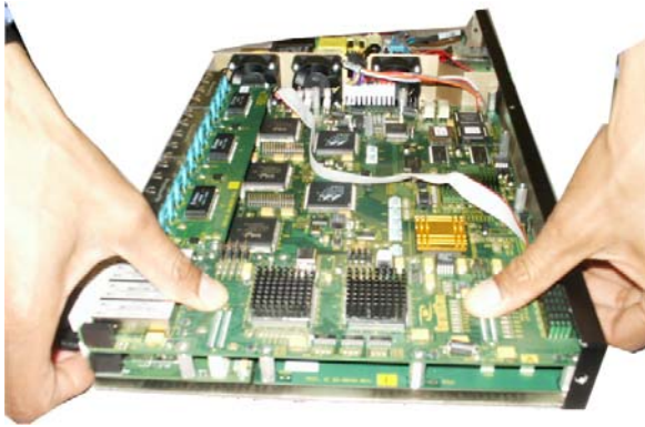
Fig.3.5.2f: Securely latching up 6KPM Cards into a Magnum 6K32T & 6K32TRC & 6K32
