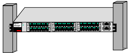
Fig 3.3.1 Dual Side-Mountings for Magnum 6K32T & 6K32TRC units
