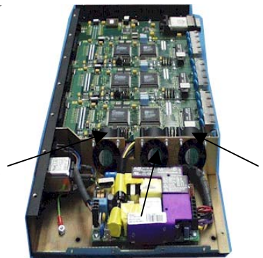
Figure 3.1: Location of the Magnum 6K32T's cooling fans
