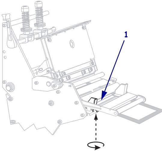
15. Push down the printhead assembly (1), and then rotate the printhead-open lever (2) clockwise until it locks into place.
