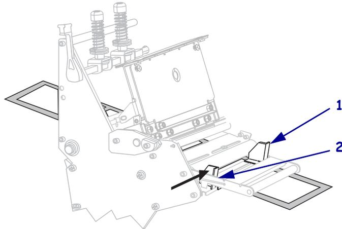
20. Tighten the thumb screw (not visible from this angle) that is located on the bottom of the outer media guide (1).
