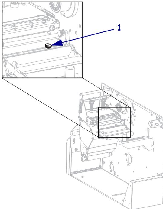
3. Using a thin, flat-blade screwdriver, loosen the upper media sensor adjustment screw.
