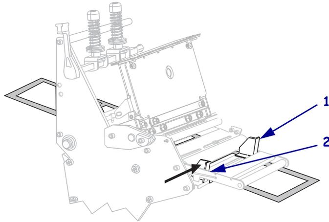
9. Tighten the thumb screw (not visible from this angle) that is located on the bottom of the outer media guide (1).
