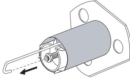
3. Slide the media or liner off of the rewind spindle.
