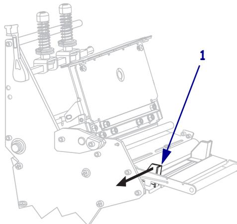
11. If your printer includes a media dancer assembly (1), thread the media under the media dancer assembly roller. For all printers, thread the media under the media guide roller (2) and then the upper media sensor (3).
