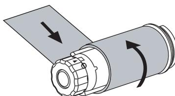
11. Rotate the spindle counterclockwise several turns to wind the ribbon and remove any slack.
