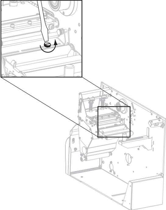
4. Slide the upper media sensor along the slot to the desired position.
