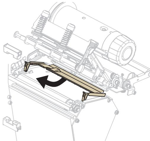
6. Using the swab from the Preventive Maintenance Kit (part number 47362), clean the back of the snap plate. In place of the Preventive Maintenance Kit, you may use a clean swab or soft cloth dipped in a solution of isopropyl alcohol (minimum 90%) and deionized water (maximum 10%). Allow the solvent to evaporate.
