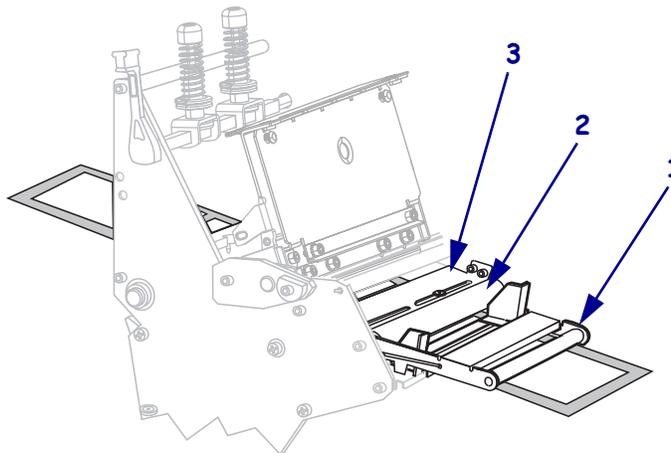
7. Push the media forward until it passes under the printhead assembly (1), under the snap plate (2), and then over the platen roller (3).
