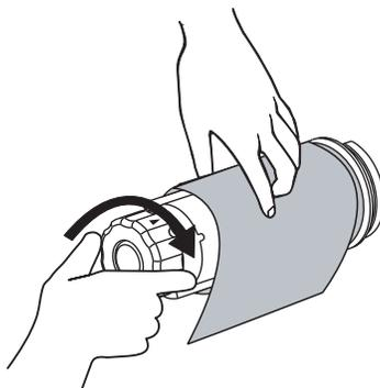
3. Slide the used ribbon off of the ribbon take-up spindle and discard.
