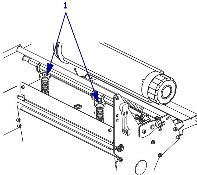
4. Some media types require higher pressure to print well. For these media types, increase or decrease pressure using the lower knurled nuts (1) until the left and right edges of the printed area are equally dark.
