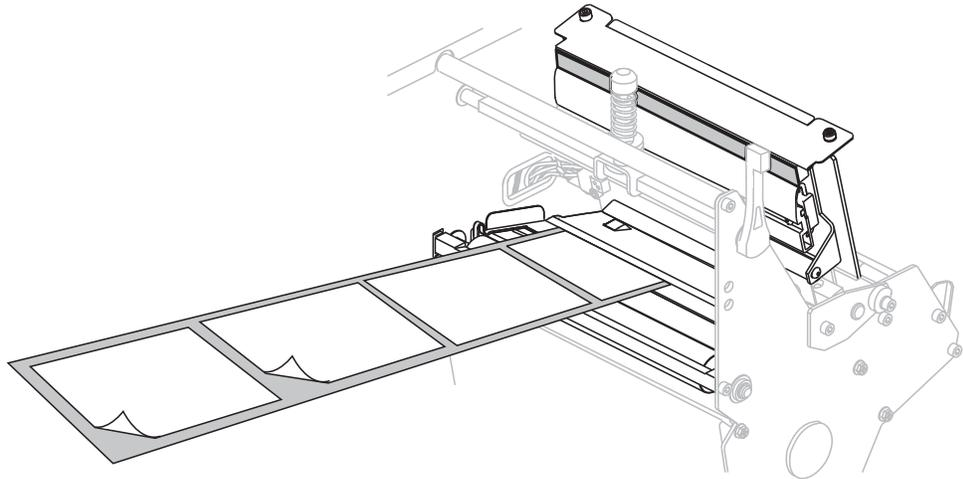
14. Remove the hook from the rewind spindle.
