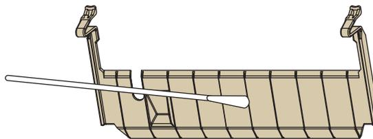
7. To reinstall the snap plate, insert the snap plate into the printer until it hits the stops (1) on the back of the encoder plate.
