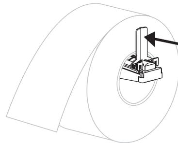
4. Continue with the media loading procedure for the desired print mode.
