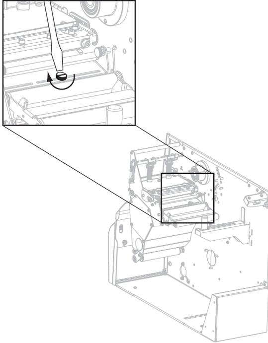
6. Adjust the lower media sensor to match the new position of the upper media sensor. See [Lower Media Sensor on page 79](#).
