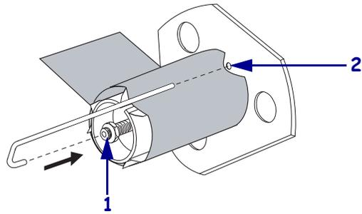
18. Rotate the spindle counterclockwise several turns to wind the media liner over the hook and remove any slack.
