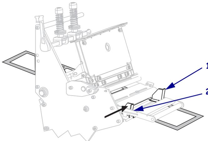
14. Tighten the thumb screw (not visible from this angle) that is located on the bottom of the outer media guide (1).
