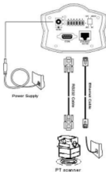
Shut down all the peripheral devices prior to connection. Connect the supplied cables from NetworKam to related devices according to the above diagram. Note that the power adaptor must be kept unplugged until other cables are firmly connected.
