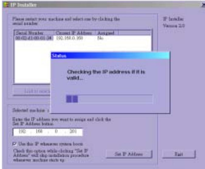
If the IP is not taken by another network device in the network, the Installer program will continue with the setup. Otherwise another message window will warn that the assigned IP conflicts. In this case, administrators should ask the network supervisor for a vacant IP address.
