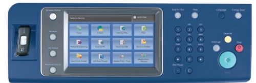
The easy-to-use touch screen interface includes a USB port option for convenient memory device connection.
