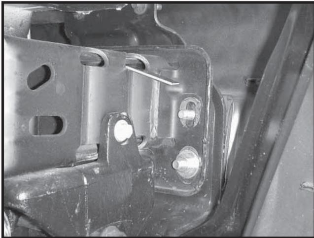
4. Insert correct side pull pod on side where bumper bolts were removed. Put two 1/2" x 1-3/4" bolts through out side edge of pod. In the back where bottom bolt comes through, use 1/2" flat washer, 1/2" lock washer, and 1/2" hex nut. Before tightening bolt, lift bumper up and center top bolt in middle of slot while holding pull pod straight. Put 1/2" flat washer, 1/2" lock washer, and 1/2" hex nut on top bolt and tighten. **NOTE:** We recommend using "LOCTITE® Blue" on all bolts
