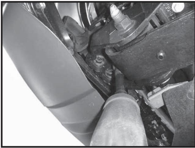
2. Pull bumper forward and remove three tow hook bolts. The tow hook or bolts will not be reused.
