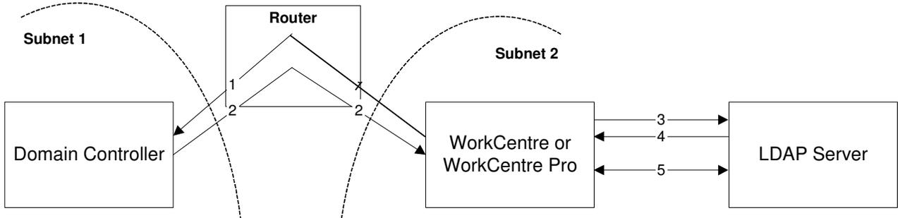
Device and Domain Controller are on different Subnets, SA defines Hostname of Domain Controller
