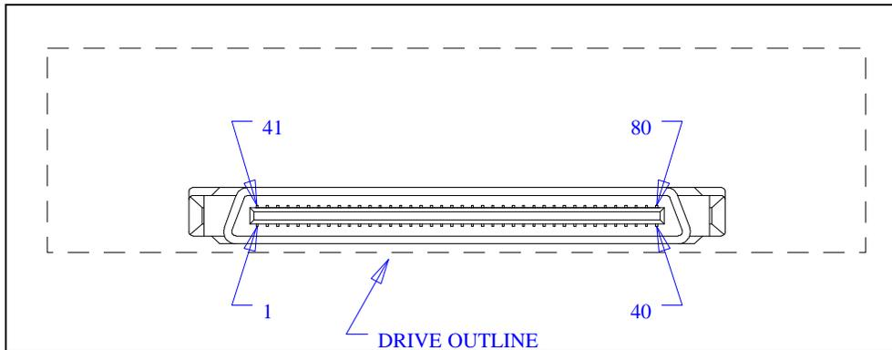
Table 6-8. 80-Pin (SCA-2) SCSI Connector Pin Assignments
