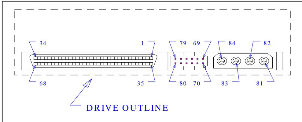
Table 6-5. 68-pin SCSI Connector Pin Assignments
