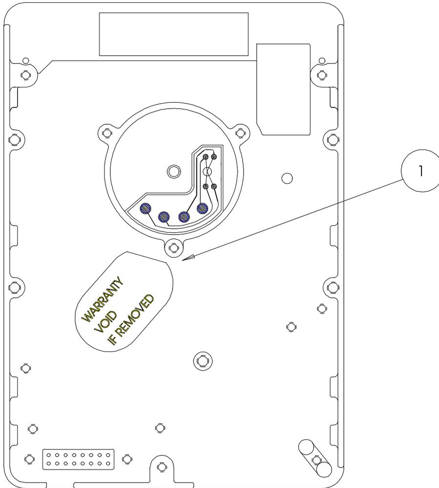
Figure 2-8. PCBA Thermocouple Locations
