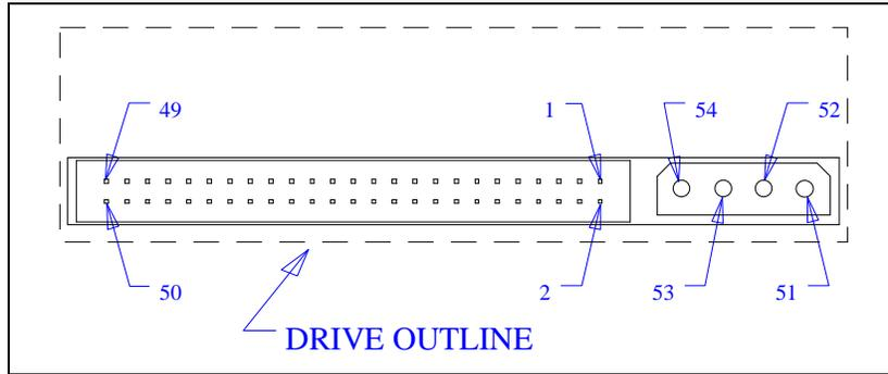
Table 6-3. 50-Pin SCSI Connector Pin Assignments
