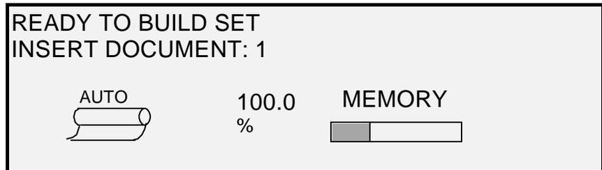
4. Insert each document of the set one at a time into the Scanner as prompted by the display. As the documents are scanned, the amount of memory used is shown in the rectangular graphical display.
