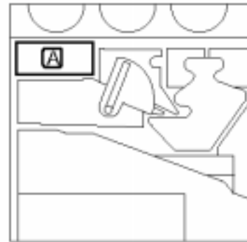
Figure 15: Locating the old Dry Ink Waste Container
