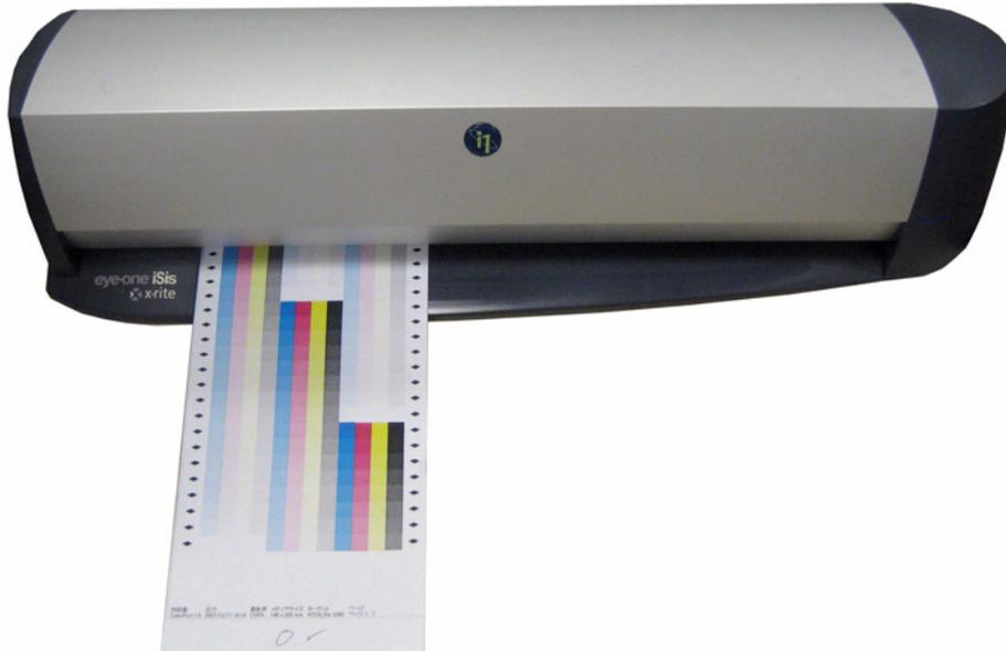
7. After the color data has been successfully processed, remove the test pattern from the Eye-One iSis and press **[OK]** at the pop-up window.
