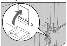
The circuit breaker is normally  $\mathbf{On}$  ("I") position, as shown in the figure. If power to the machine is interrupted, the circuit breaker trips and the switch is in the  $\mathbf{Off}$  (" $\mathbf{O}$ ") position.
