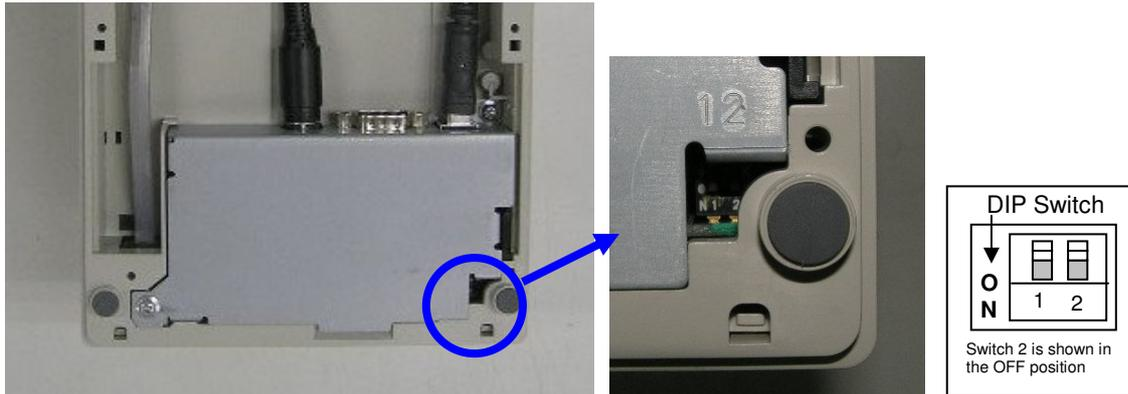
2. Power on the printer while holding the Paper Feed Button. The printer will print the Current Setting Form, then cuts the paper to print the Mfg Adjustment Menu.
