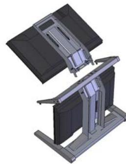
4. Thread the cables from the top monitor through the rectangular hole in the cross bracket.
