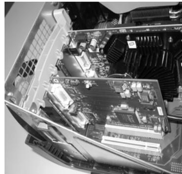
*Mirror-flip PCI card installed*
