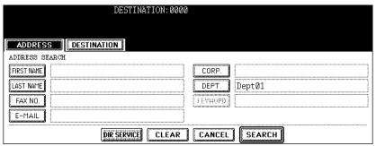
When pressing each button, the letter entry screen is displayed. Enter the value using the keyboard and digital keys, and press the [ENTER] button to set the entry.
