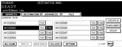
The selected contacts are displayed as reversed buttons. To cancel the selection, press the contact again, then the button will be a normal button.
