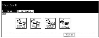
**[SCAN TO E-FILING]** — Press this to store the scanned images to e-Filing. When you store the scanned images to e-Filing, you can manage them using the e-Filing web utility. You can also retrieve them into your computer using TWAIN driver application or File Downloader.
