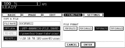
[PDF (MULTI)] — Press this to attach the scanned data as a multiple page PDF file. When scanning several pages, this equipment will store all pages as one PDF file. [PDF (SINGLE)] — Press this to attach the scanned data as a single PDF file for each page. When scanning several pages, this equipment will store each page separately as PDF files.
