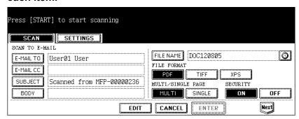
· When pressing each button, the letter entry screen is displayed. Enter the value using the keyboard and digital keys, and press the [ENTER] button to set the entry.
