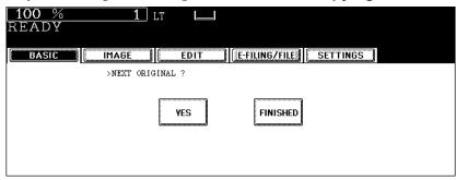
When the original is set on the Automatic Document Feeder, this screen is not displayed.
