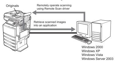
The Remote Scan driver can connect to this equipment over a TCP/IP network.
