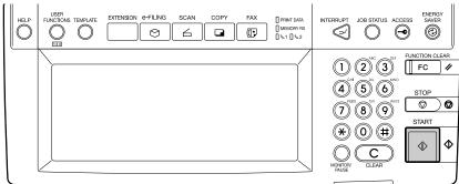
10 If the "NEXT ORIGINAL?" message is displayed, place another original on glass and press the [YES] button to copy another original, or press the [FINISHED] button to finish copying.
