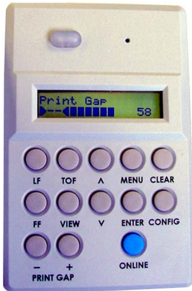
Figure 2 - 8. Typical display when adjusting Print Gap
