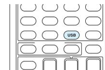
5. Connect the USB storage device to the USB port of the unit.
