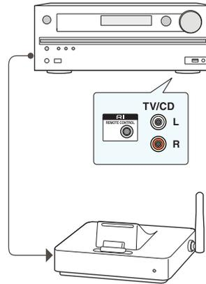
Connect an Onkyo component with RI jack to this unit using an RI cable and an analog audio (RCA) cable. For details, refer to the instruction manual of the component with RI jack. The RI cable can be connected in any order. When there are two RI jacks, both jacks work in the same way and are interchangeable.
