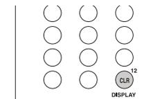
3. With the number buttons, enter the 5-digit remote control code within 30 seconds.
