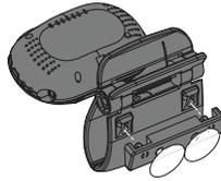
2. Firmly press the camera with the suction base attached onto glass or metallic surfaces.
