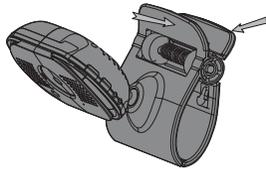
2. Place the unit over the mounting surface and release.
