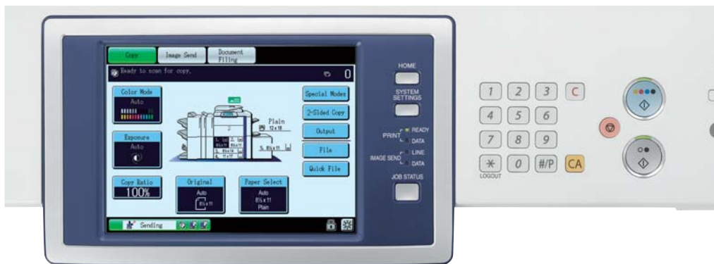
The large 10.4" (diagonally measured) Color LCD touch-screen display is intuitive and easy to use. New customizable "short-cut" keys recall frequently used documents or settings in a flash.
