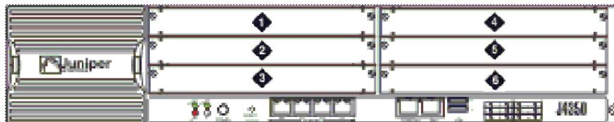
The J-series router chassis has six slots. The TGM550 can be housed in any of the six router slots. The TIMs can also be housed in any slot. Gigabit Ethernet and Fast Ethernet PIMs can be housed only in slots 3 or 6. Other optional PIMs can be housed in any slots.
