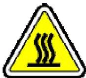
During normal operation some parts of the machine will become extremely hot. To avoid the risk of scalding please do not touch the following parts when the machine is turned on as they will be hot:
