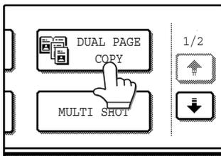
The [DUAL PAGE COPY] key is highlighted to indicate that the function is enabled, and the dual page copy icon (📄📄) will appear in the screen.
