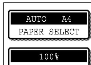
If the desired copy paper size is not selected, use the [PAPER SELECT] key to select the paper size. After the paper size is selected, touch the [AUTO IMAGE] key. A suitable ratio will be automatically selected.
