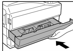
If you loaded a different size of paper that was loaded previously, place the appropriate paper size card in the front of the paper tray to indicate the new paper size.
