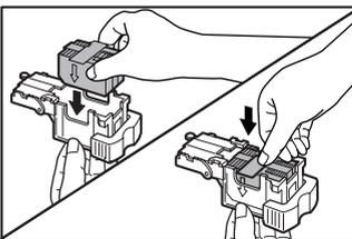
Insert the new cartridge by aligning the arrows on the cartridge with those on the box. Check that the cartridge has locked into place by pulling it slightly.
