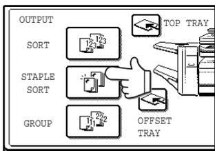
When the [STAPLE SORT] key is selected, the offset tray is automatically selected as the output tray. The top tray and centre tray cannot be used.
