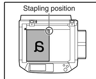
When copying B4 or A3 (8-1/2" x 14" or 11" x 17") vertically oriented originals, the copies will be stapled at the position shown below.
