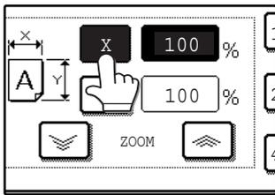
The [X] key is selected (highlighted) by default, so there is normally no need to perform this step (Go to step 5.). If the [X] key is not highlighted, perform this step.
