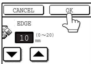
Use the ▼ and ▲ keys to adjust the erase width. The erase width can be set from 0 mm to 20 mm in increments of 1 mm (0" to 1" in increments of 1/8").
