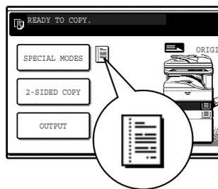
When the machine is used in copy mode or fax mode and a special mode is selected, a icon representing the feature will appear on the touch panel. If this icon is touched, the setting screen of the function (or a menu screen) will appear, allowing the settings to be checked, adjusted, or cancelled.
