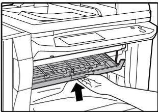
**5** If the offset tray is being used, remove any misfed paper from the offset tray.
