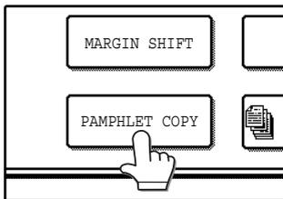
The pamphlet copy setting screen will appear. The pamphlet copy icon (📖, etc.) will also appear in the upper left corner of the screen to indicate that the function is enabled.
