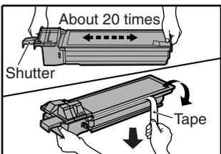
Grasp the hand grip to hold the cartridge. Do not hold the cartridge by the shutter. Be sure to only shake the cartridge before the tape is removed.
