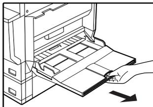
To enable correct detection of the paper size, be sure to pull out the bypass tray extension.
