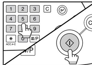
Scanning begins. When scanning of the first set of originals (A in the above example) is finished, insert the second set and press the [START] key (Ⓢ).
