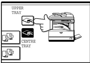
The output tray can only be selected when a job separator or finisher is installed.
