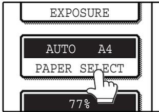
If AUTO PAPER SELECT is enabled, the appropriate copy paper size is automatically selected based on the original size and selected copy ratios.
