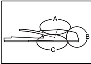
Check sections A, B, and C in the illustration at left and remove the misfed original.
