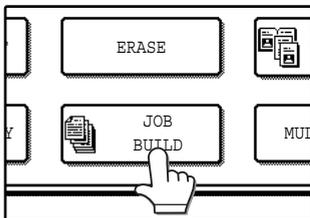
The [JOB BUILD] key is highlighted. The job build copy icon (📄) will also appear in the screen to indicate that the function is enabled.
