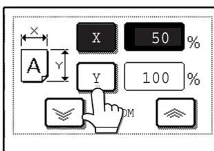
**7 Use the reduction, enlargement, and [ZOOM] keys ( [ ] / [ ] ) to change the copy ratio in the vertical (Y) direction.**
