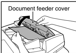
Open the document feeder cover and carefully remove the misfed original from the document feeder tray. Close the document feeder cover.
