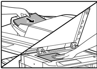
If originals are placed in the RSPF, the sort function is automatically selected. (To disable this function, see the "Key operator's guide".)
