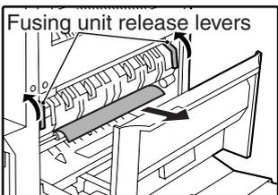
**Warning** The fusing unit is hot. Do not touch the fusing unit when removing misfed paper. Doing so may cause a burn or injury.
