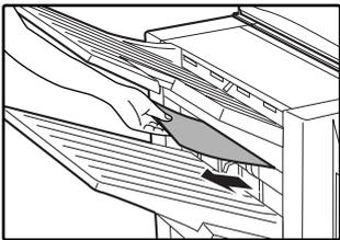
**6** If the top tray is being used, open the top cover, remove any misfed paper, and close the top cover.
