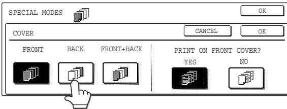
To add only a front cover, touch the [FRONT] key. To add only a back cover, touch the [BACK] key. To add both a front and back cover, touch the [FRONT+BACK] key.
