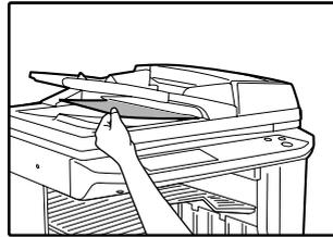
Carefully remove the misfed original from the exit area.
