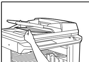
If the misfed original cannot be removed, open the document transport cover (below), and rotate the release roller again.
