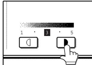
If [TEXT] was selected for the original image type, touch the [AUTO ◀▶ MANUAL] key to select [MANUAL] and then adjust the copy exposure.
