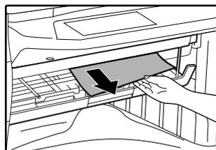
**3** If staple sort copying is being performed, open the paper guide and remove any misfed paper from the stapler compiler.
