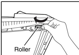
Open the RSPF and rotate the release roller in the direction of the arrow to feed the original out. Close the RSPF and then carefully remove the original.
