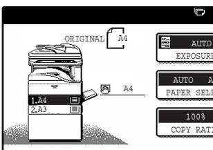
The selected tray is highlighted. If the tray contains a different size of paper than the original, "LOAD xxxx PAPER." will appear.
