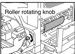
**4 Lift the fusing unit release levers and carefully remove the misfed paper.**
