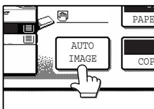
A suitable ratio is selected based on the original size and selected paper size. (The ratio appears in the touch panel.)
