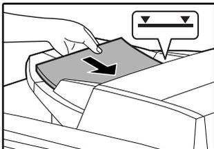
Insert the originals all the way into the feed slot. The original size appears in the touch panel.
