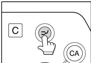
The [INTERRUPT] key (⊖) blinks until the machine is ready for the interrupt job, after which it lights steadily.
