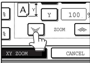
The [ZOOM] keys ( [ ] / [ ] ) can be used to change the ratio in increments of 1%. Touch the [ ] key to increase the ratio, or the [ ] key to decrease the ratio. Continuing to touch a [ZOOM] key ( [ ] / [ ] ) makes the ratio change faster.
