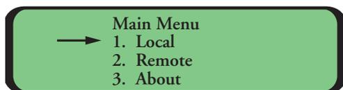
Use the "up" and "down" buttons to move the cursor to "1. Local". Press the "enter" key to select the Local Menu:
