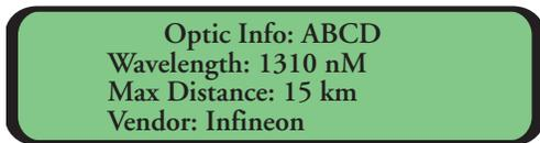
The Info Menu shows the wavelength (normally 1310nM), maximum distance (normally 15km) and optic transceiver vendor name (Infineon) for the selected optic transceiver. Use the "+" button to select the next transceiver. Use the "-" button to select the previous transceiver.
