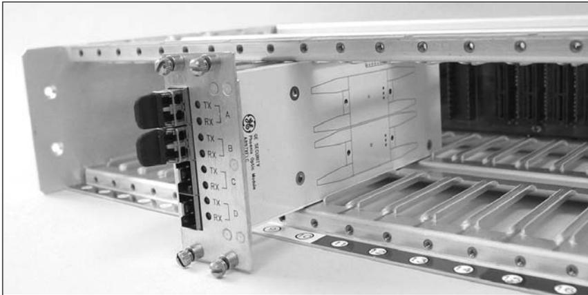
**INSERT OPTICAL TRANSCEIVER MODULES IN SLOTS 9-10 (White)**
