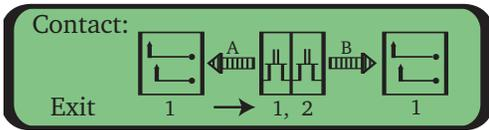
Please refer to the Video Input Mapping Menu described earlier for important notes regarding channel mapping and instructions on how to enable mappings. However, note that contact signals are mapped as pairs since there are 8 contact channels per Contact Closure Module.
