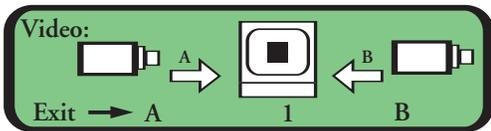
Press "+" and "-" to select an output channel while the cursor is under the middle icon. Use "left" and "right" to move the cursor at the bottom of the screen. To enable fiber port A move the cursor to the left and then press "enter." Similarly, to select fiber B, move the cursor to the right and press "enter." To leave this screen move the pointer to "Exit" and press "enter." All channel mapping are saved when you leave this menu.
