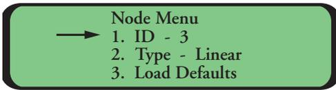
Every Phoenix node (i.e. chassis) in a system must have a unique node ID number. The node ID is set to zero the first time a Phoenix chassis is switched on, or if you Load Defaults. Zero is an invalid node ID; it must be a number between 1 and 255. Once set, the node ID will be remembered if the chassis loses power.
