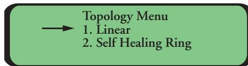
In order for a Phoenix chassis to route information over its fiber links correctly, it must know the topology of the entire system. A chassis can be part of either a Linear or Self-Healing Ring topology. If you are configuring a Self-Healing Ring topology, then each node must also know the total length of optical fiber used in the ring. Once set, the topology will be remembered if power to the chassis is lost.
