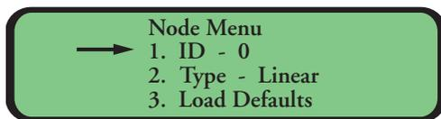
If you are configuring a system with a linear topology, and item 2 in the menu reads, "2. Type - Linear", then you do not have to make any changes and can continue to Step 3, below. Otherwise, select item 2 from the menu. This displays the Topology Menu:
