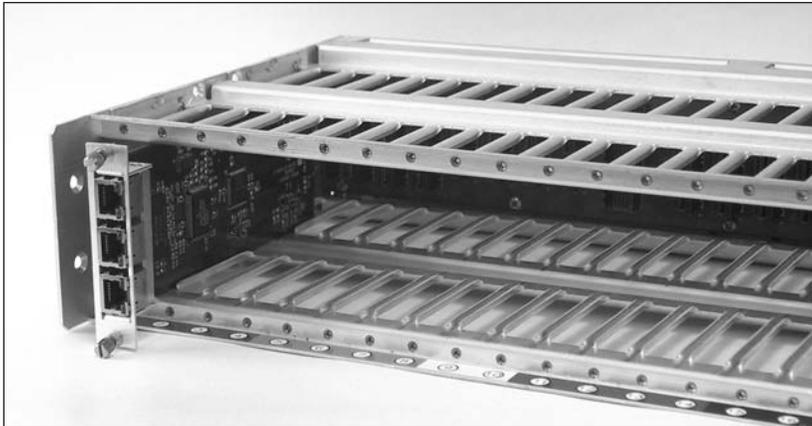
INSERT ETHERNET MODULES IN SLOTS 1-4 (Red)
