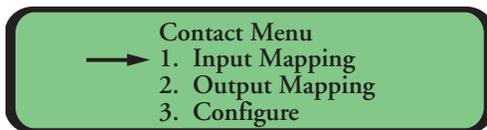
Contacts Input and Contacts Output channel mapping, monitoring, and configuration can be accessed from the sub-menus.
