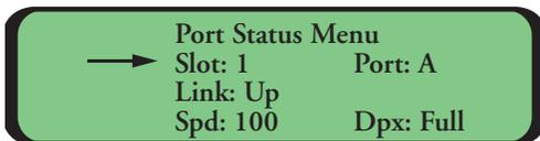
This screen allows you to monitor the link status of each port of an Ethernet module. Use the arrow keys to move back and forth between the slot and port selections. The '+' and '-' buttons increment and decrement the slot and port selections. Port A is the top port, Port B is the middle port and Port C is the bottom port. The link status is indicated as either Up or Down. If the Link is up, the negotiated speed and duplex are indicated. Press 'enter' to leave this menu.
