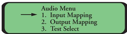
Audio Input and Audio Output mapping and tests can be accessed from the sub-menus.
