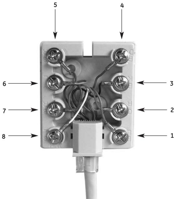
Figure 2. RJ45 Socket
