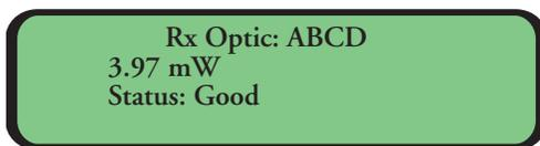
This screen shows the optical receive power of the selected optic transceiver. Use the "+" button to select the next transceiver. Use the "-" button to select the previous transceiver.
