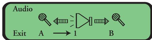
This screen allows you to select which optic port is being reviewed for each of the 16 audio output channels. The number under the speaker icon indicates which audio channel is selected. The letters under the microphone icons indicate at which optic port the selected output channel will be looking. Arrows to the left and right of the speaker icon indicate that the mapping is enabled. If the output channel is not mapped to a fiber then the corresponding arrow is not shown.
