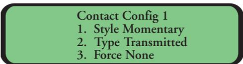
This menu allows the user to change the format or test a specified contact channel. Use "+" and "-" to change selections at each line in the menu. Press "left" to exit this screen. The top line of this menu shows the currently selected channel. The second line, "1. Style" shows the current contact format:
