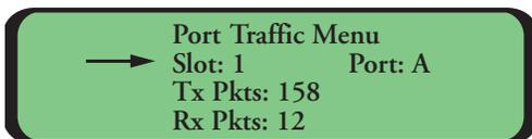
This screen allows you to monitor the number of error-free packets sent and received at each port of an Ethernet module. The '+' and '-' buttons increment and decrement the slot and port selections. Port A is the top port, Port B is the middle port and Port C is the bottom port. The packet counters wrap around to 0 once they reach 65,535. Press 'enter' to leave this menu.
