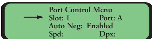
This screen allows you to control the link parameters for each port of an Ethernet module. Use the arrow keys to navigate around the screen. The '+' and '-' buttons increment and decrement the slot and port selections, and toggle the Auto-Negotiation, Speed and Duplex settings. Port A is the top port, Port B is the middle port and Port C is the bottom port. Port A is the top port, Port B is the middle port and Port C is the bottom port. Press 'enter' to leave this menu.
