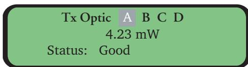
This screen shows the optical launch power of the selected optic transceiver. Use the "+" button to select the next transceiver. Use the "-" button to select the previous transceiver.
