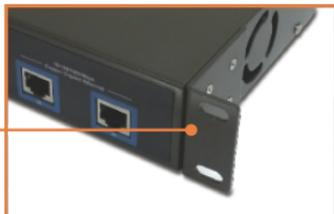
4. Carefully position the switch onto the rack. Align the bracket to the screw holes on the rack, then use the screws provided with the equipment rack to mount the switch.
