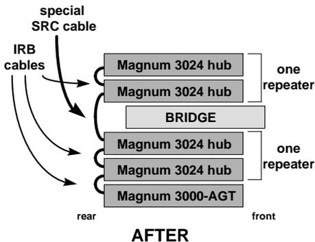
The same result could also be achieved by installing a Magnum Bridge Port Module (BPM) into the Bonus Port of one of the repeaters and connecting it to a port on the other repeater.
