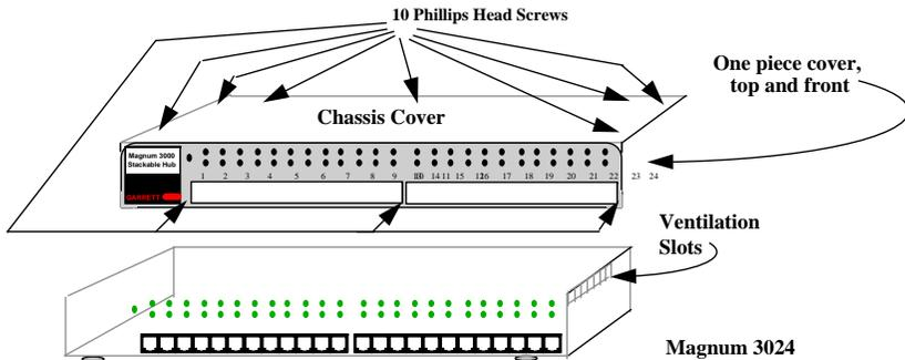
Figure 5.3a: Removing Magnum 3024 / 3012 Chassis Cover
