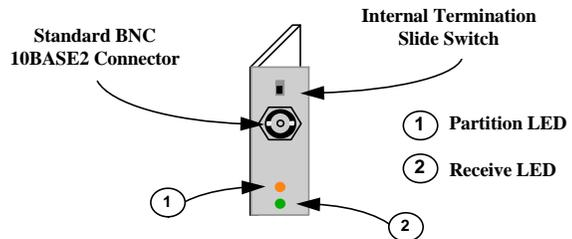
**Important Note:** for the RPM-BNC Termination Switch - DOWN (or right) = Internally Terminated, UP (or left) = "T" Connector required.
