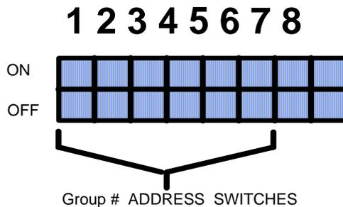
Figure 2.3.3a, Group # Address Switches, Enlarged Illustration
