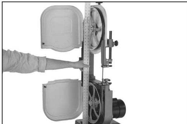
**Figure 68.** Checking if the wheels are coplanar.
