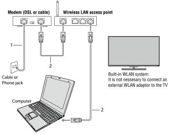
(Sample Illustration) L9300UC Series—Connecting with Internet connection - wireless
