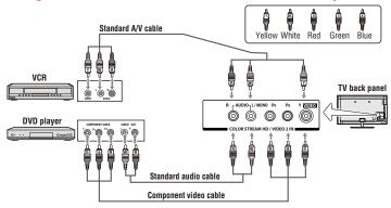
(Sample Illustration) L9300UC Series—Connecting a DVD with ColorStream® or a VCR with composite video
