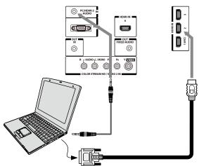
(Sample Illustration) L9300UC Series—Connecting to an HDMI<sup>™</sup> terminal
