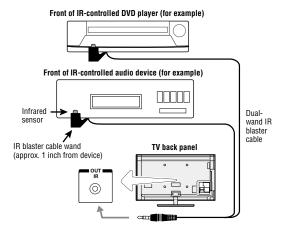
(Sample Illustration) L9300UC Series—Using the IR blaster OUT terminal
