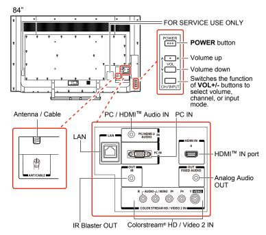
(Sample Illustration) L9300UC Series back panel controls and connections
