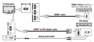
(Sample Illustration) L9300UC Series—Connecting an HDMI<sup>TM</sup> or DVI device to the HDMI<sup>TM</sup> Input
