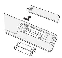
(Sample Illustration) Removing the battery cover
