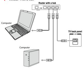
(Sample Illustration) L9300UC Series—Connecting a network without Internet connection
