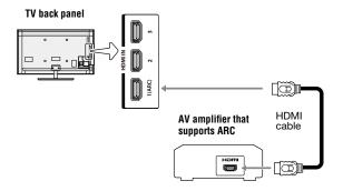
(Sample Illustration) L9300UC Series— Connecting to HDMI™ ARC
