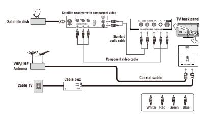
(Sample Illustration) L9300UC Series—Connecting to an antenna, satellite receiver, and/or cable TV box
