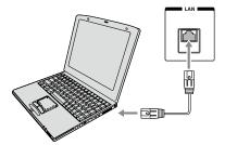
(Sample Illustration) L9300UC Series—Connecting a computer without Internet connection
