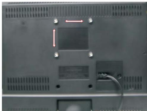
Mounting Specification : **75mm x 75mm** using screw size **M4**. Length of screw should not exceed **6mm**. Please Note : The **6mm** length of screw refers to how deep the screw can go inside the mounting holes. When you're buying screws, you should add the original 8mm to the thickness of your mounting plate in order to get the total screw length.
