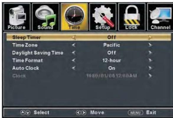
2. Press “▲/▼” button to select “Time Zone” and press the “◀/▶” button to enter time zone adjustment menu to select the local time zone.
