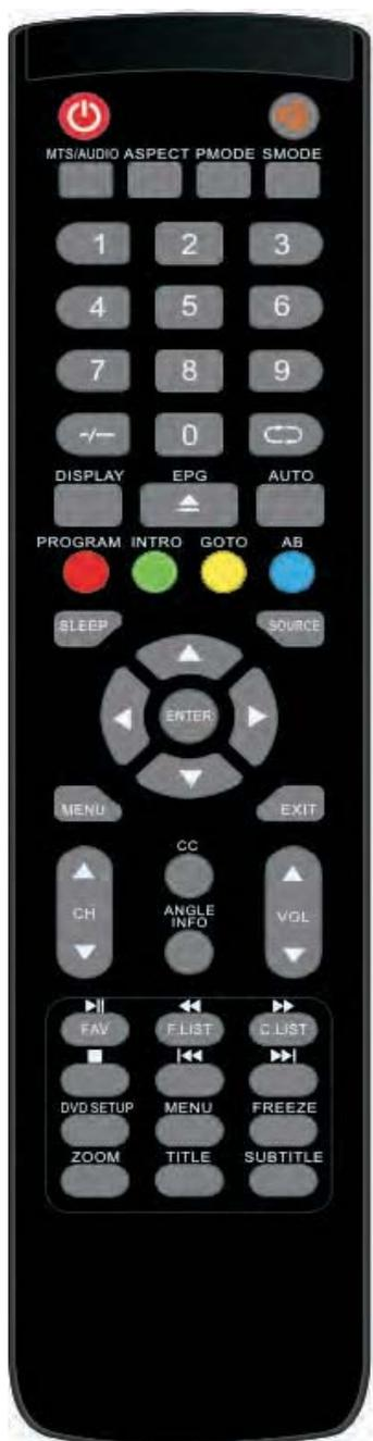
**Power** : Press this button to switch on the TV when at standby mode or enter standby mode.
