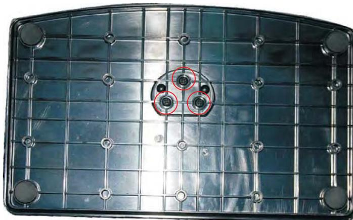
2.To remove the stand, remove the 2 screws in the area and the stand will come off.
