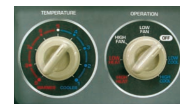
Manual Control Panel
