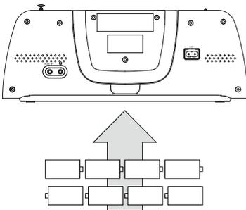
The unit can also be powered by batteries. (Requires 8 C size batteries, not included).
