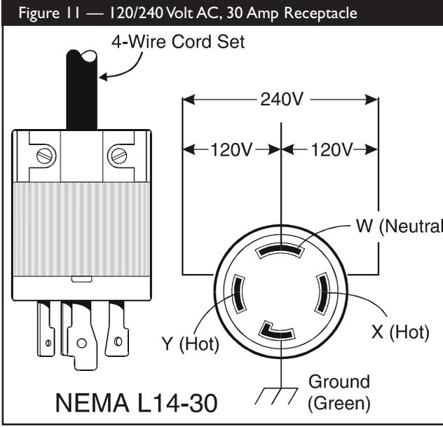
This receptacle powers 120/240 Volt AC, 60 Hz, single phase loads requiring up to 3,600 watts of power (3.6 kW) at 30 Amps for 120 Volts OR 7,000 watts of power (7.0 kW) at 29.2 Amps for 240 Volts. The outlet is protected by a 30 Amp push-to-reset circuit breaker.
