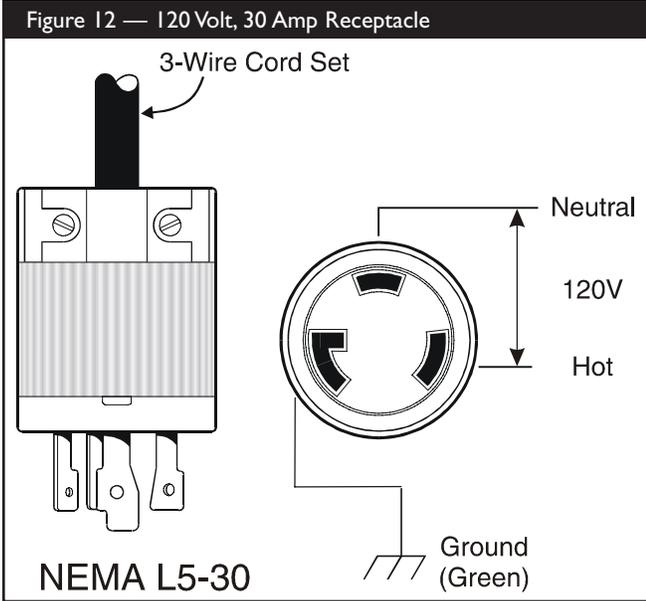
Use this receptacle to operate 120 Volt AC, 60 Hz, single phase loads requiring up to 3,600 watts (3.6 kW) of power at 30 Amps. The outlet is protected by a 30 Amp push-to-reset circuit breaker.
