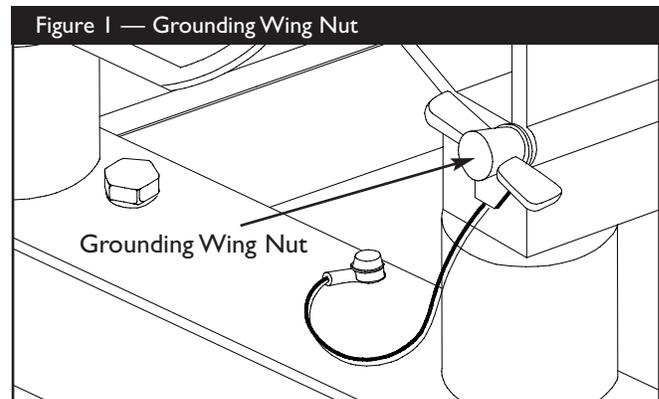
Generally, connecting a No. 12 AWG (American Wire Gauge) stranded copper wire to the grounding wing nut and to an earth-driven copper or brass grounding rod (electrode) provides adequate protection against electrical shock. Be careful to keep the grounding wire attached after connecting the stranded copper wire. However, local codes may vary widely. Consult with a local electrician for grounding requirements in your area.
