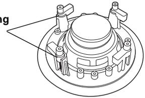
To remove the speaker from the wall or ceiling, loosen the screws only far enough to remove the speaker. This will prevent loss of the mounting tabs.
