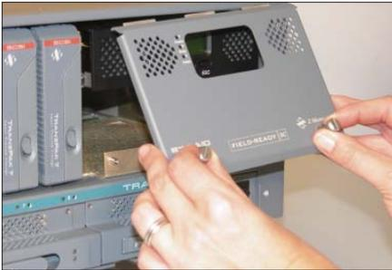
The door can be removed by lifting it down and off of the hinge.
