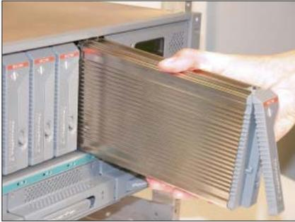
With the handle in the open position, hold the TranzPak 7 by the main body and insert it partially into the docking bay. ( Be sure that it is sliding on the black guides).
