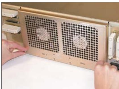
Seat the assembly down and secure it in place by simultaneously pressing and turning the thumbscrews clockwise. Tighten the thumbscrews.
