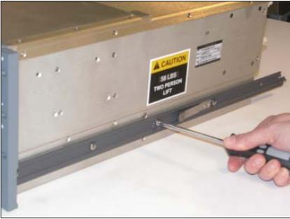
**CAUTION:** When attaching the inner members of the slide assemblies to the sides of the 8X RAID, ensure screw penetration does not exceed 3/16" length. Damage may result if screw length exceeds 3/16" length. Use 10-32 x 3/16" screws only (part# 01-91827).
