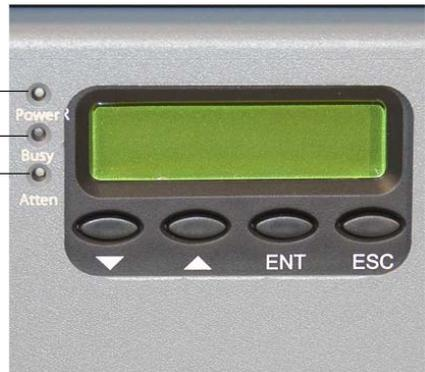
The System Power Indicator= illuminates when power to the system is detected.
