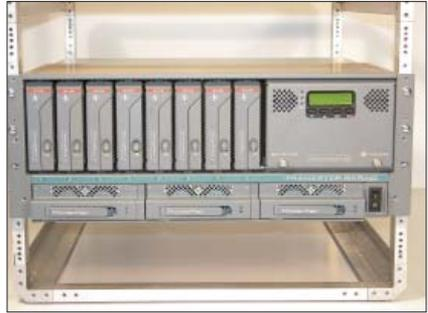
until it snaps the locking handle in place. Check that all TranzPak 7 disk modules are aligned across the face of the 8X.
