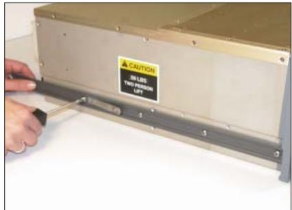
Attach the inner members to the sides of the 8X RAID using 10-32 x 3/16" panhead Phillips head screws (part# 01-91827).
