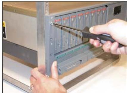
Secure the front of the 8X RAID to the rack with three 8-32 x .75" panhead Phillips screws on each side. See image above.
