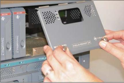
To install the controller door, seat the hinges up into the hinge slots at a 45 degree angle.
