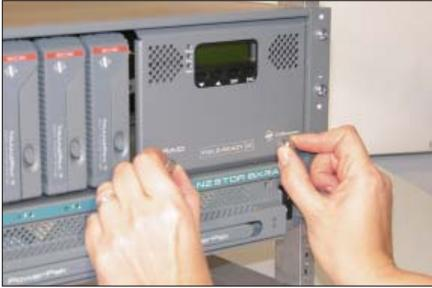
To remove the controller door, turn the thumbscrews on the face of the door counterclockwise.
