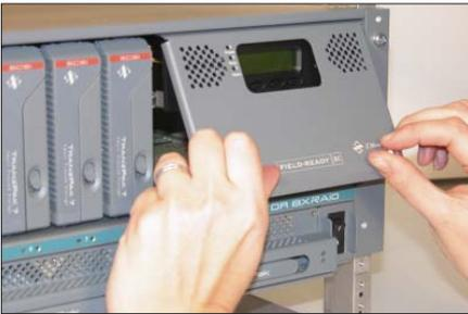
Rotate the bottom of the door down to align the thumbscrews with the screw holes.
