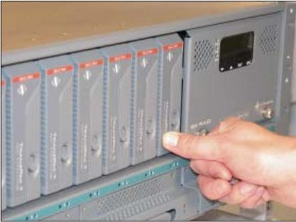
Check that the locking catch is aligned with the locking indent in the slide rail and press the handle towards body...
