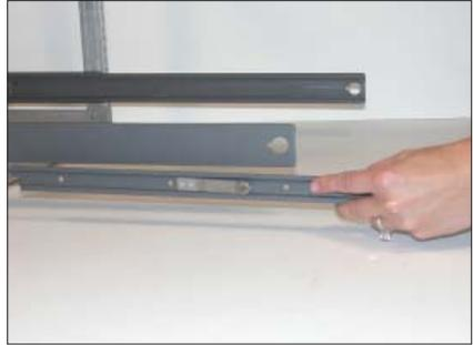
and remove the inner members of the slide assemblies.
