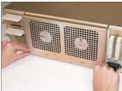
With your fingers, turn the two thumbscrews (locations shown above) counter clockwise until the screws loosen.
