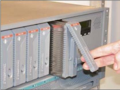
Pull handle gently forward to eject the TranzPak 7 off of the rear connector.
