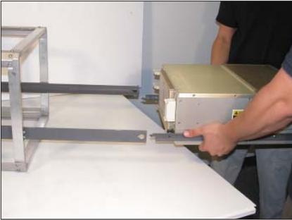
Hold the 8X RAID up to the extended rails with the rear of the 8X RAID to the rear of the rack. Insert the inner member (attached to the 8X RAID) into the middle member of the slide.
