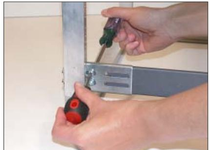
Tighten the slide assembly screws using a Phillips screwdriver and 3/8" ratchet. Repeat rail installation for other side.
