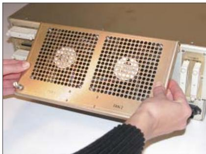
To install the new fan assembly, place the two hinges into the hinge slots (shown in the next photo) at a 45 degree angle.
