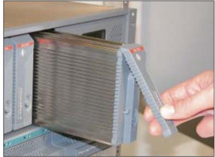
Continue to gently pull handle to slide the TranzPak 7 forward. The TranzPak 7 should slide over the grounding contacts until it is half way out.
