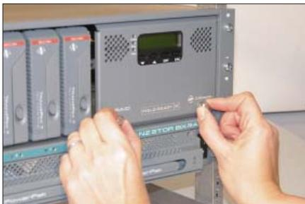
Simultaneously press and turn the thumbscrews on the face of the door clockwise. Tighten the thumbscrews.
