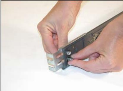
Insert the screws through the slots of the extension bracket and into the holes in the outer slide member. Secure loosely with flat and lock washers. Do not tighten. Repeat with the second slide assembly.
