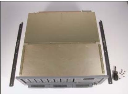
Lay the inner members along either side of the 8X RAID, placing the pointed end of the members toward the rear of the unit. This is how the inner members will be attached to the 8X RAID.
