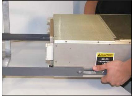
Slide the unit in until the slide action stops.
