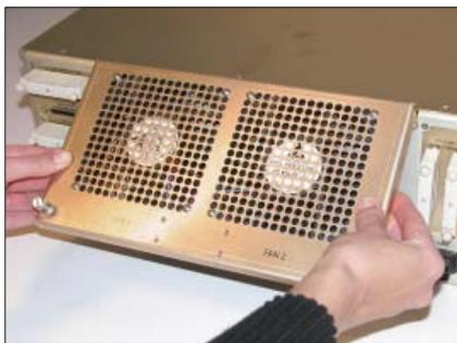
Rotate the fan assembly upward on the hinge and then down.
