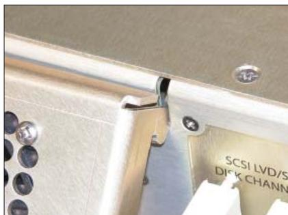
The image above shows a hinge being inserted into the hinge slot.
