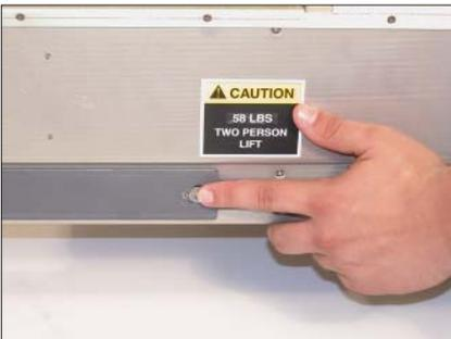
Simultaneously press the slide locking tab in and push the unit all the way back into the rack.
