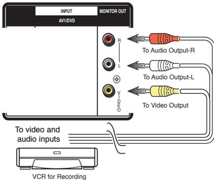
The picture signal being displayed on the TV screen is output through the Monitor Output Jacks. Use these terminals to record TV broadcasts and for video dubbing from AV1 or AV2 input terminals.
