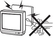
High voltages are used in the operation of this television receiver. Do not remove the cabinet back from your set. Refer servicing to qualified service personnel.
