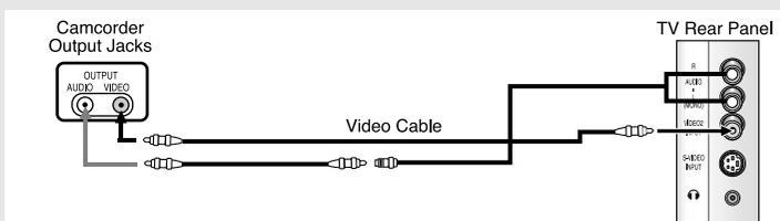
The audio-video cables shown here are usually included with a Camcorder. (If not, check your local electronics store.) If your camcorder is stereo, you need to connect a set of two cables.
