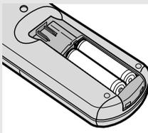
◀ Make sure to match the “+” and “-” ends of the batteries with the diagram inside the compartment.
