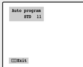
◀ The TV automatically cycles through all of the available channels and stores them in memory. This takes about one to two minutes. Press **MENU** at any time to interrupt the memorization process and return to the Channel menu.
