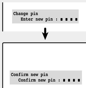
As soon as the 4 digits are entered, the "Confirm new pin" screen appears. Re-enter the same 4 digits. When the Confirm screen disappears, your PIN has been memorized. Press **MENU** three times to exit.
