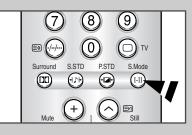
The "S.Mode" button displays/controls the processing and output of the audio signal. When power is switched on, the mode is automatically preset to either "Dual-I" or "Stereo", depending on the current transmission.
