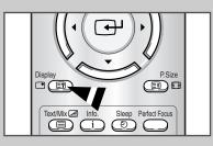
You can set the television's clock so that the current time is displayed by pressing the "DISPLAY" button. You must also set the time if you wish to use the automatic on or off timers.
