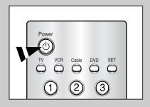
Your television can be placed in Standby mode, in order to reduce the power consumption.
