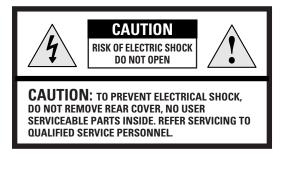
WARNING: TO PREVENT DAMAGE WHICH MAY RESULT IN FIRE OR SHOCK HAZARD. DO NOT EXPOSE THIS APPLIANCE TO RAIN OR MOISTURE. The lightning flash and arrow head within the triangle is a warning sign alerting you of "dangerous voltage" inside the product.
