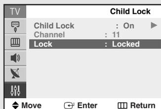
◀ If any channel is locked, you can not access to the "Channel" and "Child Lock" menu by using the control buttons on the TV panel (the "Not Available" is displayed in the "Child Lock" menu). You can access by using the remote control only.
