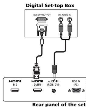
1. Connect the DVI output of the digital set-top box to the **HDMI/DVI IN1** port on the set.
