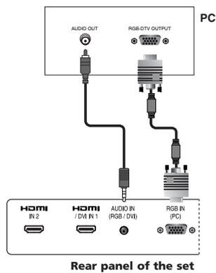
1. Connect the RGB output of the PC to the **RGB IN (PC)** port on the set.
