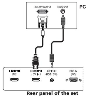
1. Connect the DVI Output on the PC to the **HDMI/DVI IN1** Input port on the TV.
