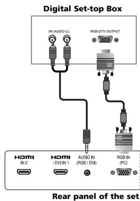
1. Connect the **RGB** output of the digital set-top box to the **RGB IN (PC)** port on the set.
