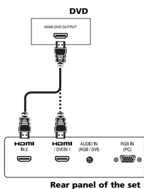
1. Connect the **HDMI** output of the DVD to the **HDMI/DVI IN1** or **HDMI IN2** port on the set.
