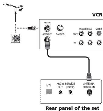
1. Connect the Antenna out socket of the VCR to the Antenna input socket on the TV.
