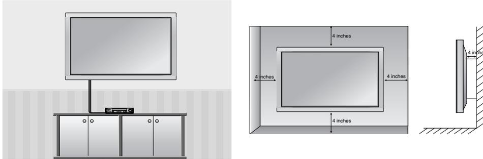
The set can be installed on a wall as shown above.
