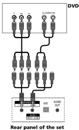
1. Connect the video outputs (Y, Pb, Pr) of the DVD to the **COMPONENT VIDEO (Y, Pb, Pr)** port on the set.
