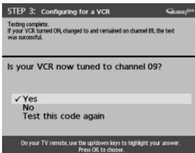
4. Look at the front display of your VCR. If your VCR turned on automatically and changed to channel 09, the test was successful. Highlight *Yes* and press OK.
