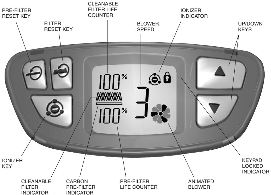
**Fig. 3 - Air Purifier Control Area and Alpha-numeric Display**
