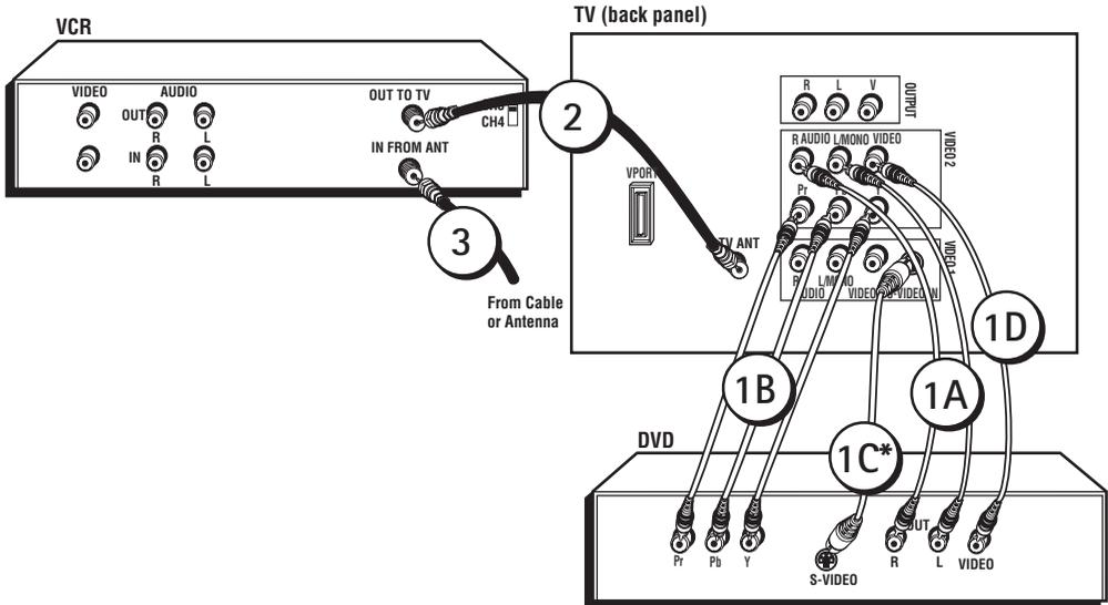
\* If you connect an S-Video cable, you must connect the audio cables to the VIDEO 1 AUDIO jacks on the back of the TV, not the VIDEO 2 AUDIO jacks.
