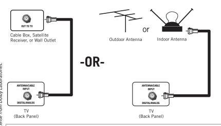
Connect your TV to cable; a cable box or satellite receiver; or an antenna in order to receive TV channels. Connect the cables as shown in the first or second connection.
